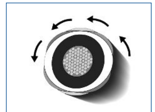
THE EFFECTS ON A WIRE AFTER RE-TWISTING WHERE BEADS HAVE BECOME FLATSPOTTED
